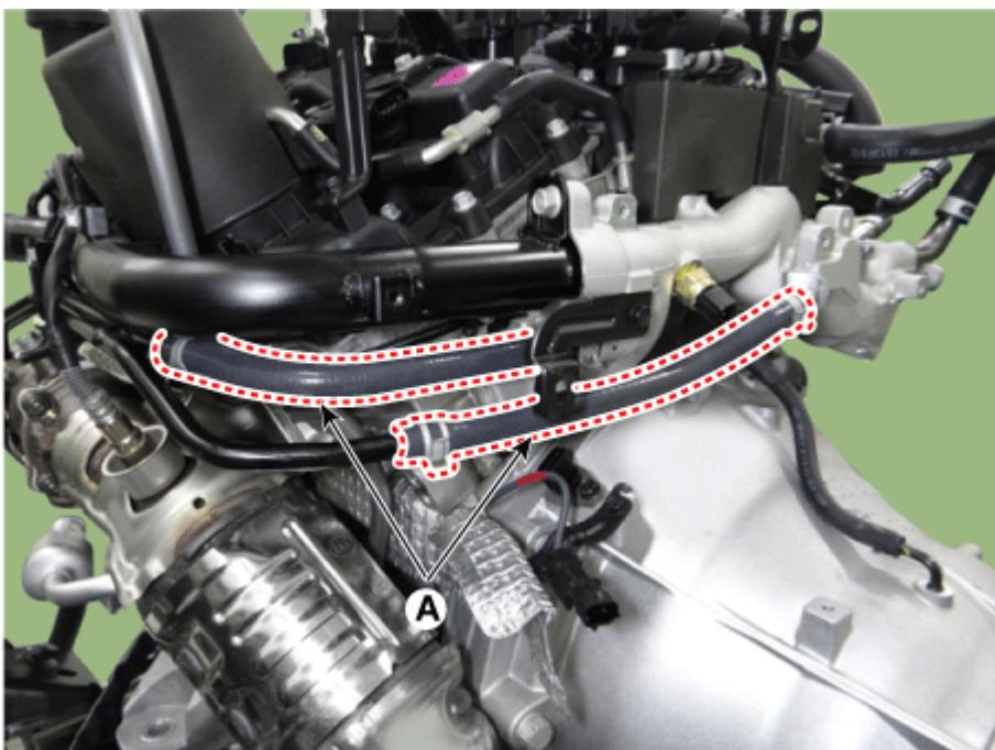
9. Remove the LH turbocharger water pipe (A).
