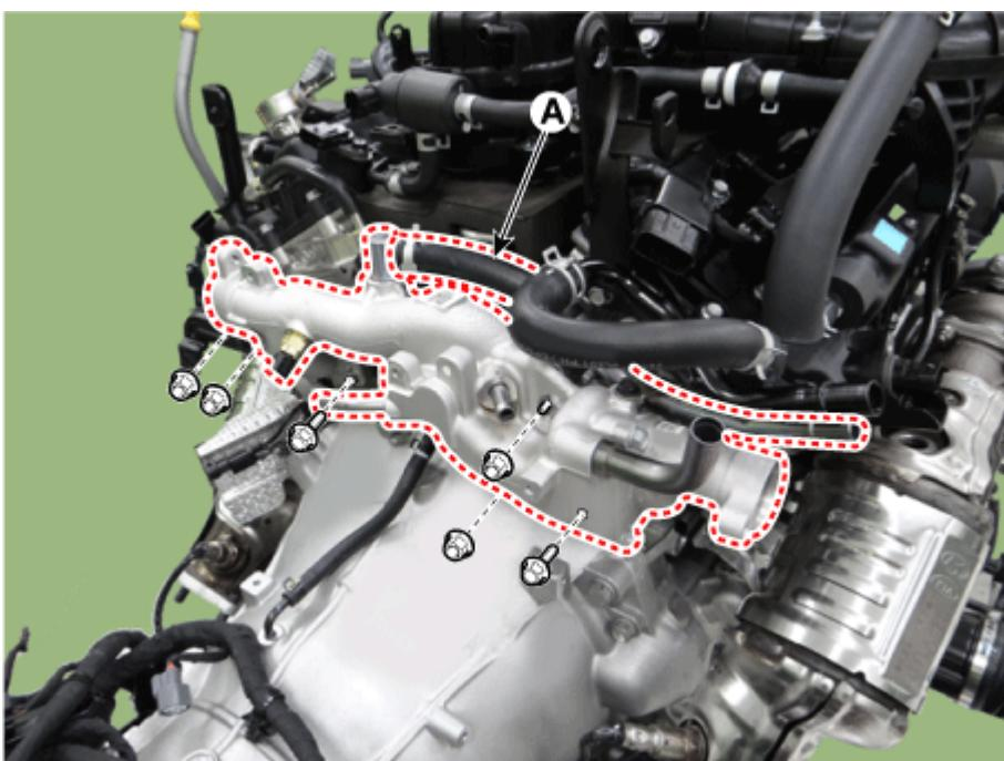
15. Remove the water temperature control assembly gasket (A).
