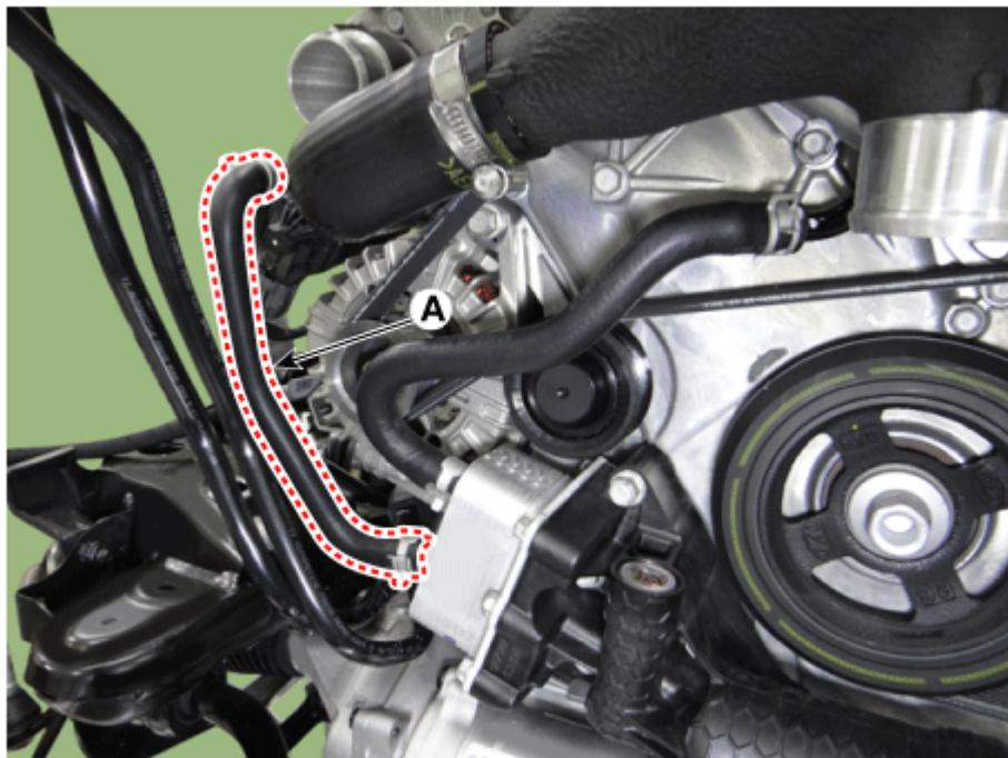
5. Remove the RH turbocharger water pipe (A).
