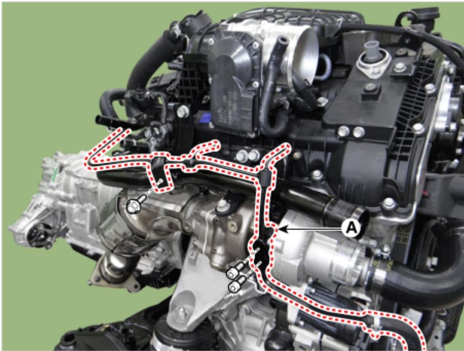
6. Remove the water inlet pipe (A).
