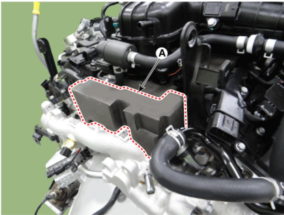
14. Remove the water temperature control assembly (A).
