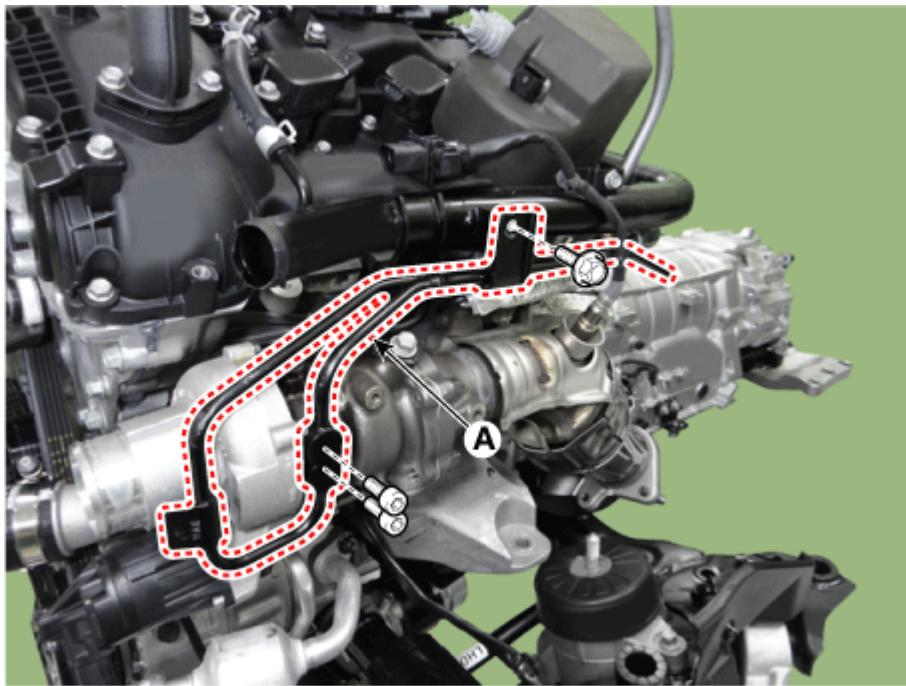
10. Remove the heated oxygen sensor (HO2S) wiring bracket (A) and heated oxygen sensor (HO2S) connector (B) from the water outlet pipe.
