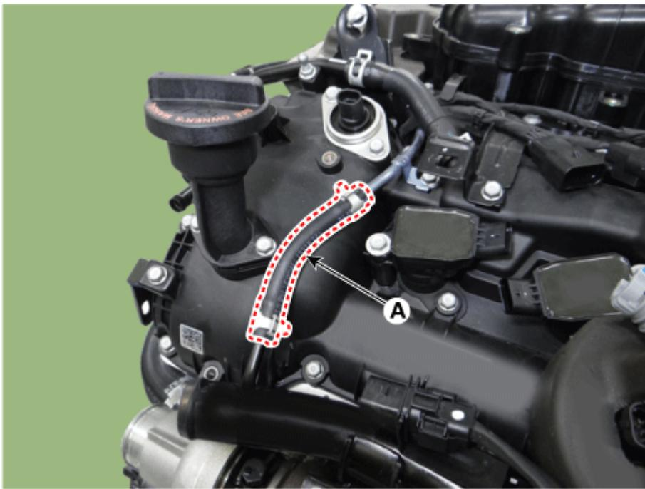
12. Remove the water outlet pipe (A).
