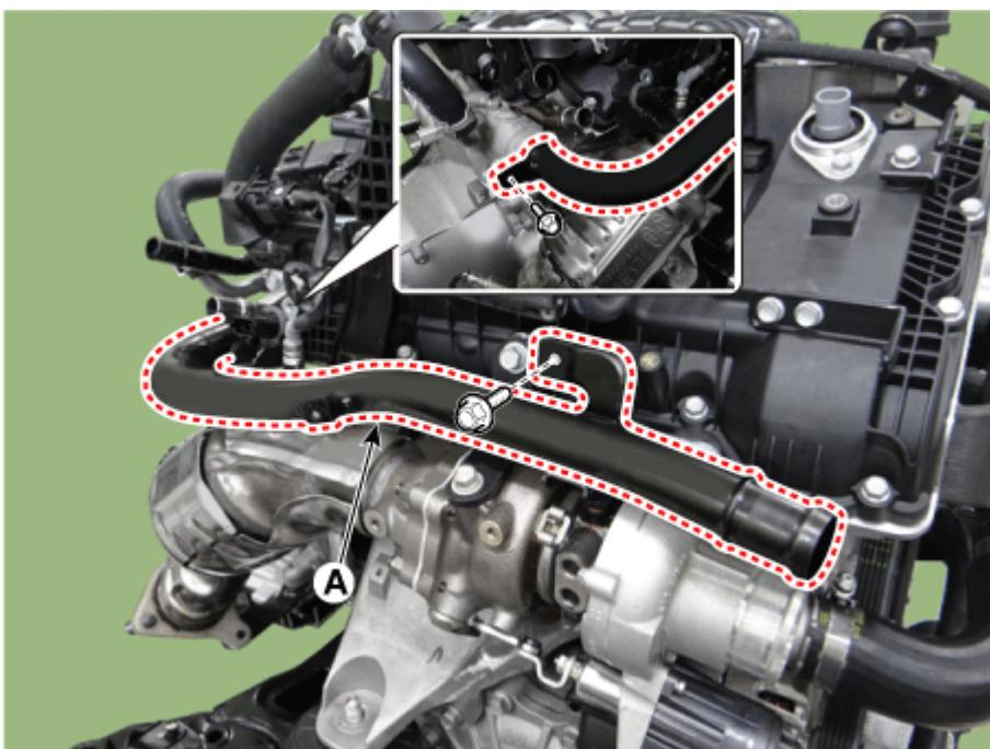
7. Remove the brake vacuum pipe mounting bolt (A).
